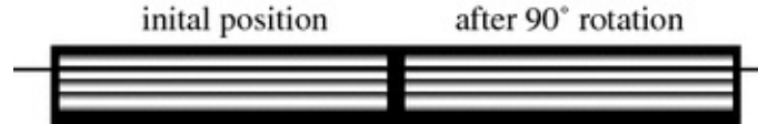
Fig. 6.5 The interference fringes before and after the rotation of 90^\circ of the apparatus
